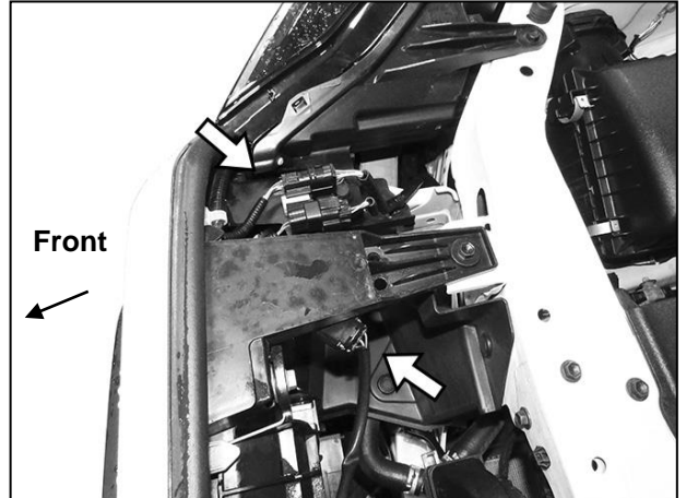
(Fig 6) Unplug all wiring harnesses leading to front bumper (passenger/right side pictured)
