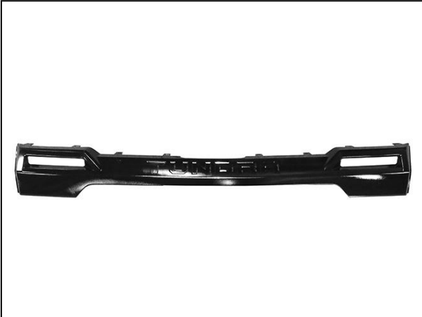
(Fig 5) Remove center body panel (fascia)
