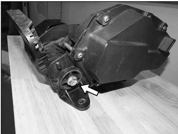
(Fig 14) Remove long pivot bolt (arrow)
