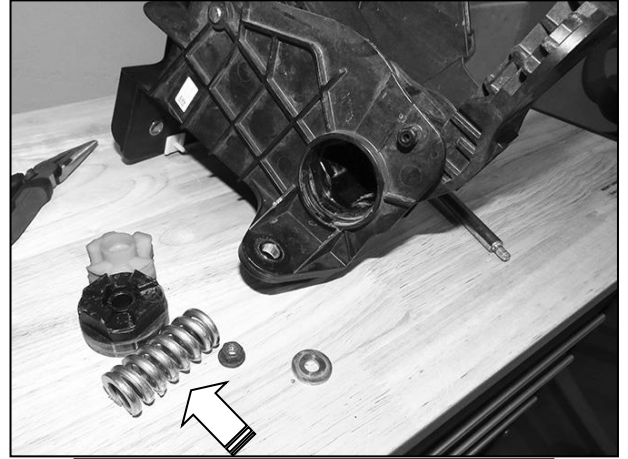
(Fig 16) Remove inner drive spring
