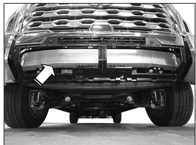
(Fig 4) Remove lower cover from bumper
