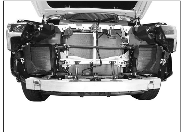
(Fig 8) Grille/bumper cover assembly removed
