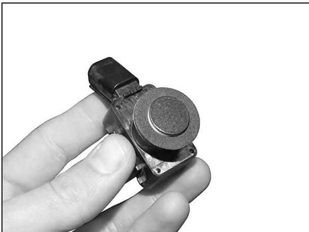
(Fig 47) Apply Foam Seals to end of sensors
