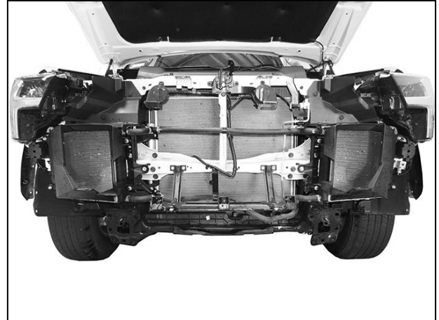
(Fig 11) Bumper, grille and impact bumper removed
