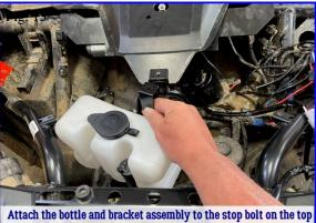
Attach the bottle and bracket assembly to the stop bolt on the top and the round bar on the bottom using the ruber coated strap.
