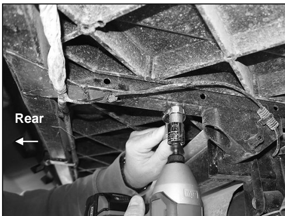
(Fig 5) Insert installation pictured, impact tool use is optional
