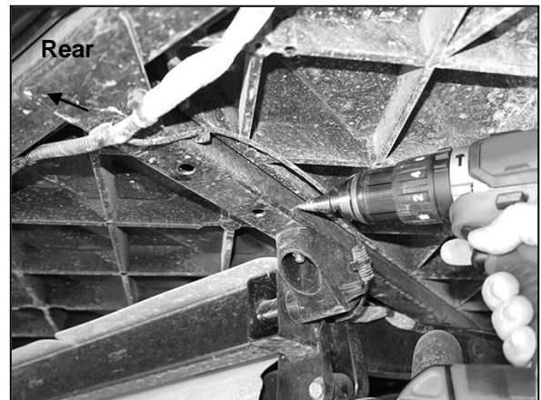
(Fig 2) Use a 5/16" drill bit to open up horizontal holes through sides of frame
