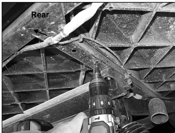
(Fig 3) Use a 7/16" drill bit to open up the (2) holes in the bottom of the frame. IMPORTANT: DO NOT Drill through frame and into bed, only enlarge the (2) bottom holes for Threaded Inserts.
