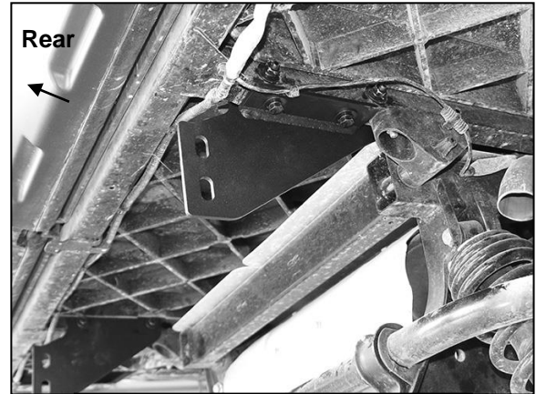
(Fig 9) Frame Brackets installed
