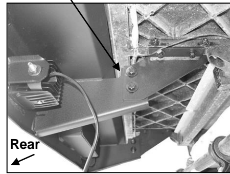
(Fig 11) Bumper installed. Attach Light to tab on back of Bumper (light not included)
