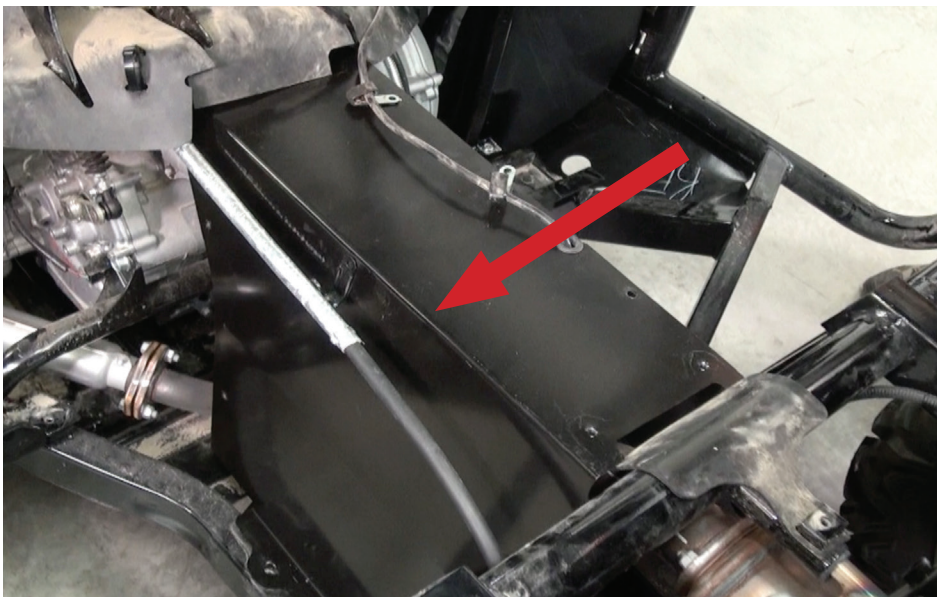
Fig 16 - Remove the driver side and top piece of exhaust tunnel. (one solid piece)
