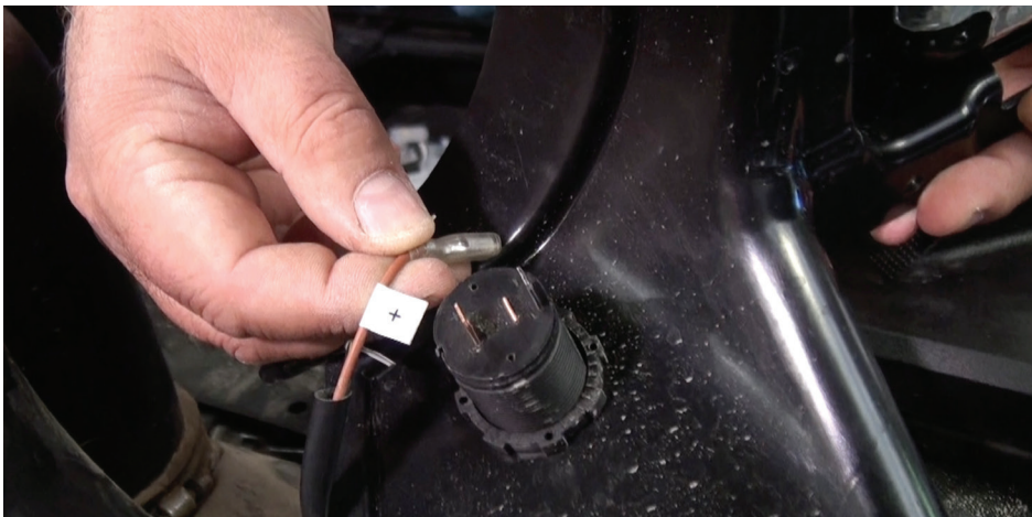
Fig. 8 remove 2 wires from accessory outlet. They are wired + & - and need to be reattached correctly later
