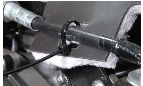
Fig 22 - Secure driver side through slots with zip tie
