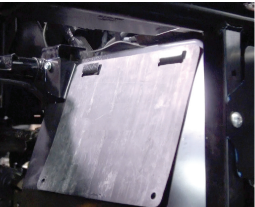
Fig 13 - Remove metal heat shield under drivers seat. The piece with the rubber flap attached to it
