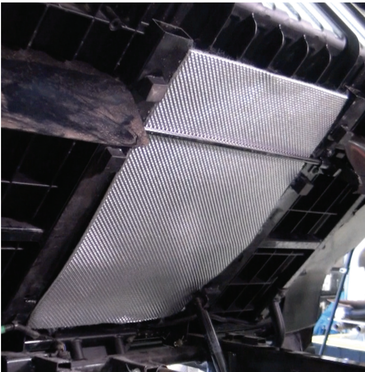
Fig 24 - Slide shield between bed and bed release bar
