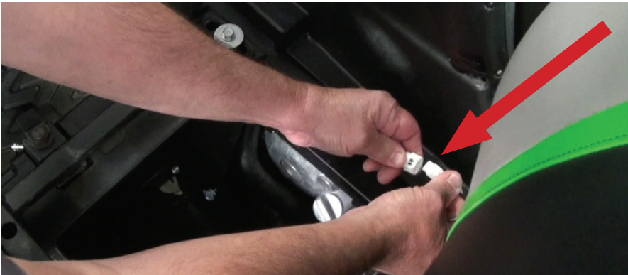
Fig. 1 - Remove driver seat bottom and disconnect seat belt warning connector
