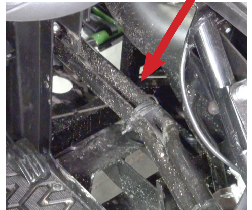
Fig 20 - Wrap these lines. Make sure hook and loop closure is facing away from exhaust
