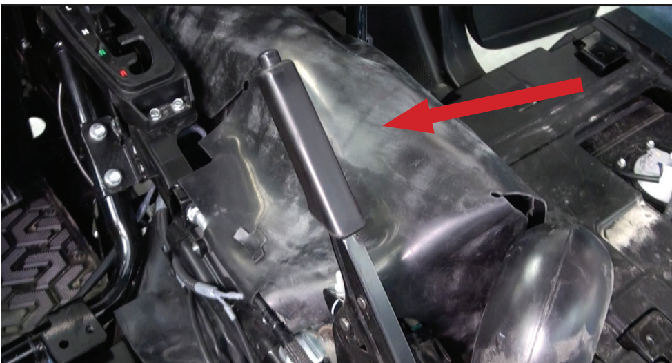
Fig 11 - Remove rubber mat on top of engine. This will not be re-used
