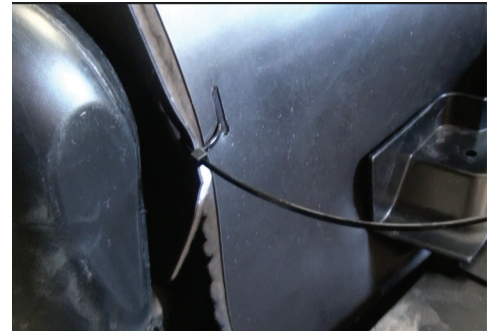
Fig 23 - Secure rear through slots with zip tie
