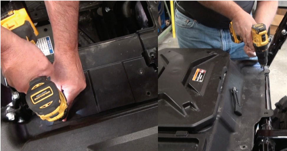
Fig. 9 - longer phillips head screws in front
