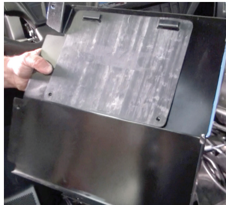
Fig 13 - Remove metal heat shield under drivers seat. The piece with the rubber flap attached to it
