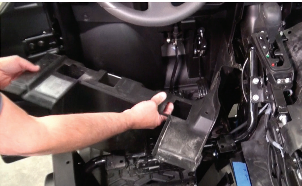
Fig. 5 - Remove all push pins on the top, front and side of trim panel under the driver seat. This piece extends all the way to the firewall in the foot well.
