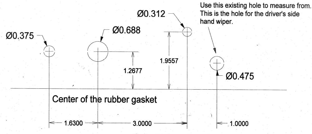
If using this for a drill template check the scale before drilling. The 1" dimension should be 1" when you measure it.
